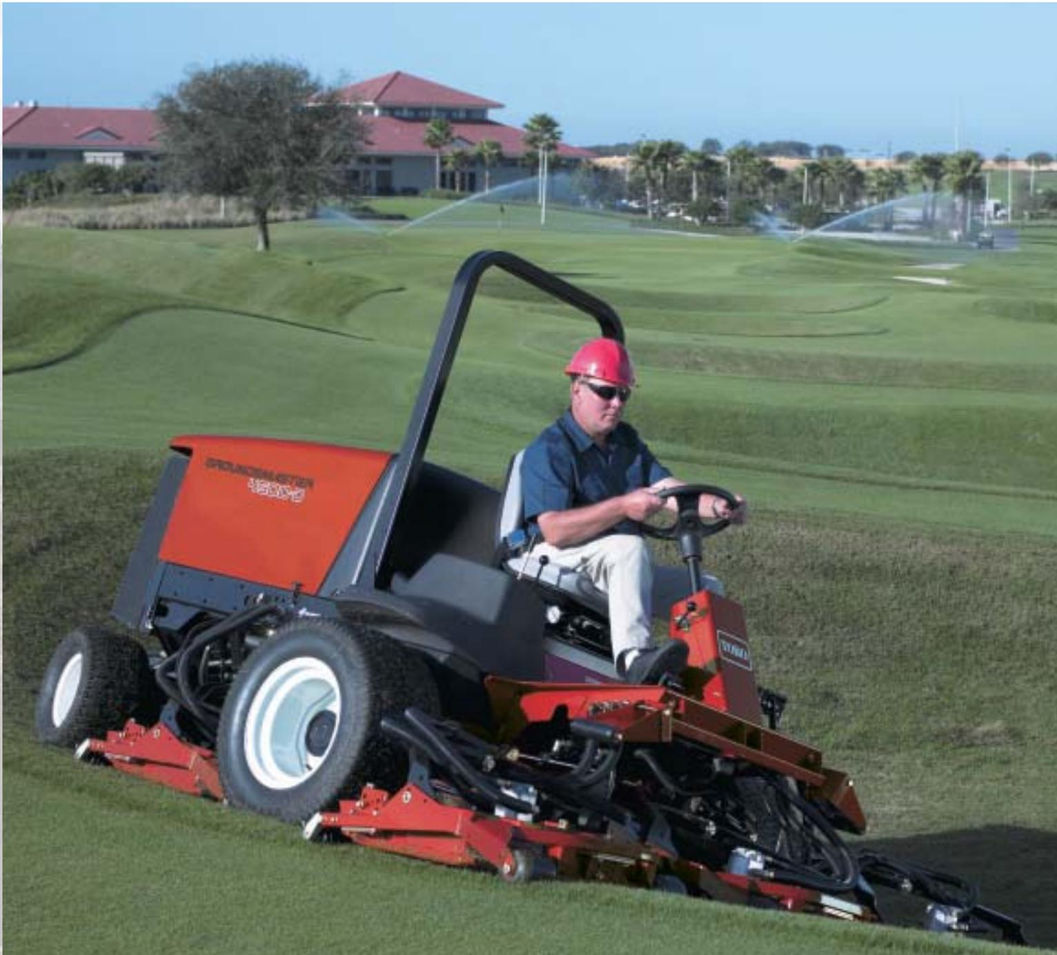
**ALL-WHEEL TRACTION** Parallel hydraulic flow between the front and rear wheels ensures solid footing at all four wheels. The bi-directional, hydrostatic drive maintains consistent traction, even on hills or wet turf. And the individual wheel brakes provide extra traction assistance when needed.
