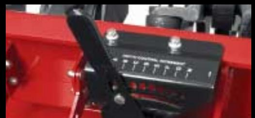
Tine depth is adjustable down to an industry-leading 4" deep (10.2 cm).
