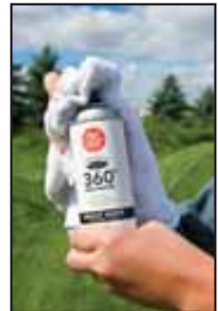
5. Place rag over nozzle and press to clear excess paint from nozzle after each hole is painted.
