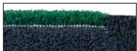
Turf heatbonded to the base.
