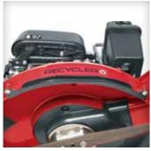
**STEEL DECK WEAR PLATE** Extend the life of your mower deck with replaceable steel wear plates that protect against bottom and side impacts. Select models.
